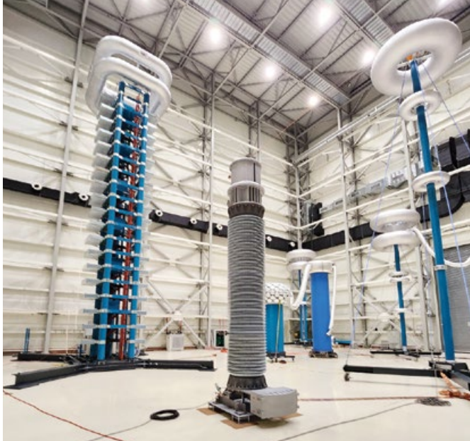
High-power voltage transformers 525 kV for US market
